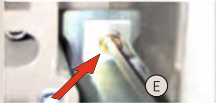
Tighten to 6Nm (4.42ft-lbs) Fest anschrauben mit 6Nm Serrare a 6 Nm (4.42ft-lbs)
