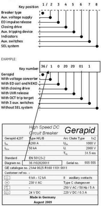
Fig. 22 Example code shown on the nameplate.
