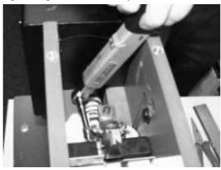
Fig. 52-6 Tighten braid's screws with torque of 10Nm
