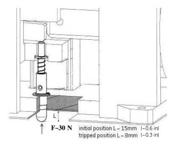
Fig. 10a Forced tripping release
