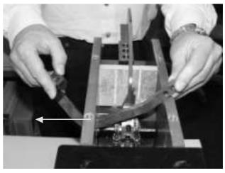
Fig. 51 Taking out the front arc runner of old design
