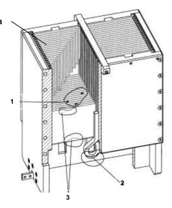
Fig. 42 Inspection of the arc chute
