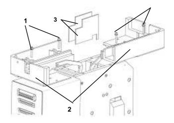
Fig. 48 Adapter and protective walls
