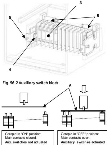
Fig. 56-3 Actuating plate for auxiliary switch block
