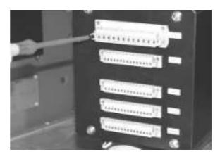
Fig. 55-1 Unscrew and remove all the external plugs
