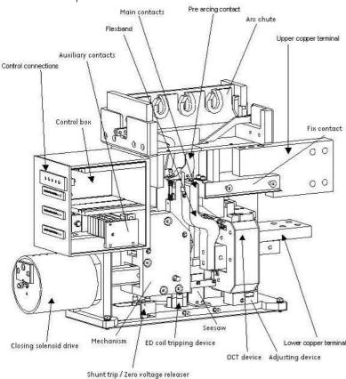
Fig. 4 Modular construction overview
