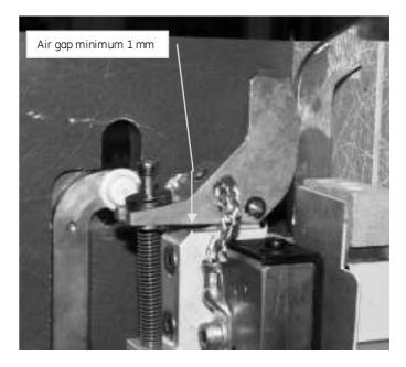
Fig. 47 Inspection of the arcing contact's air gap
