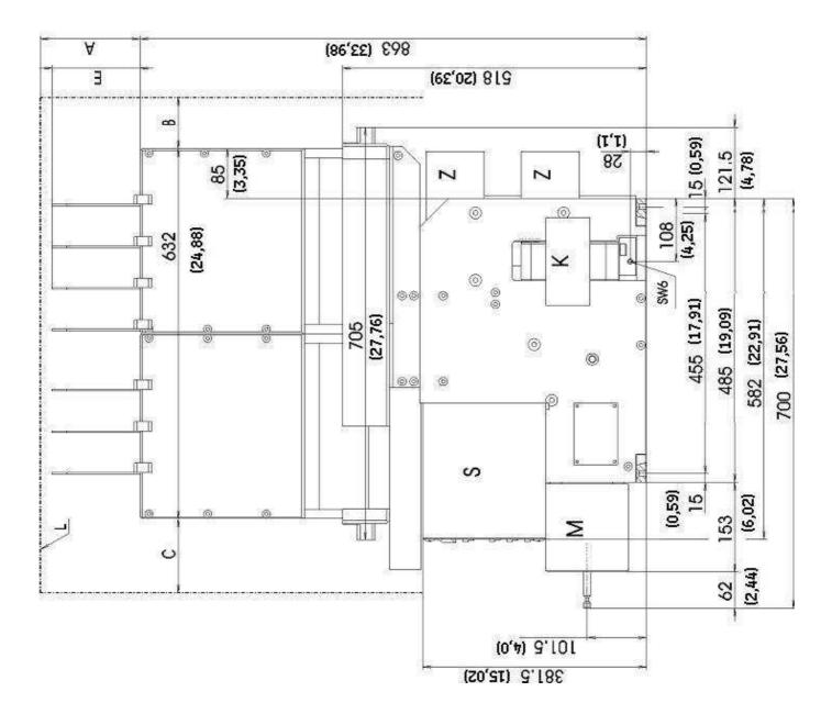
Fig. 35 Gerapid 8007 with arc chute 2x (dimensions in mm and inches)
