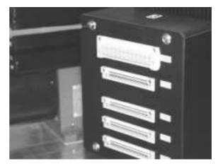
Fig. 55-2 Unscrew four bolts of the box cover
