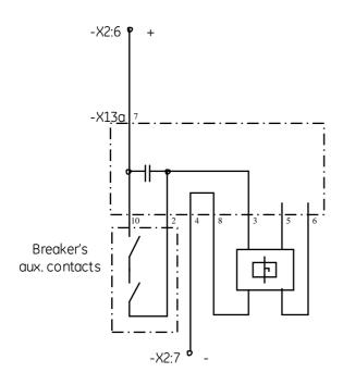
Below, non-standard shunt trip with double winding, directly supplied from external DC voltage.
