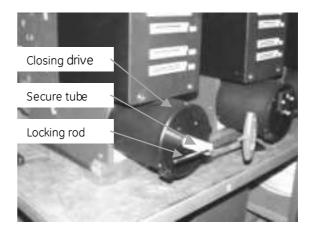
Fig. b Securing dosing drive against opening
