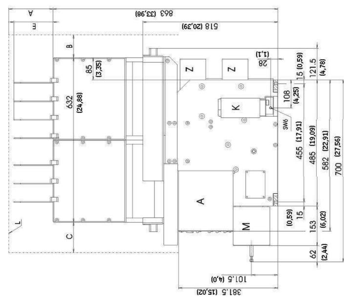
Fig. 33 Gerapid 2607-6007, arc chute 2x (dimensions in mm and inches)
