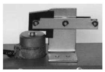
Fig. 8 EDimpulse coil with seesaw interface
