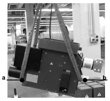
Fig. 1 Handling the breaker
