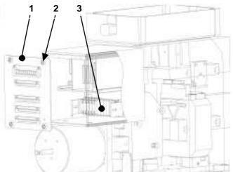
Fig. 56-1 Control box with auxiliary switch block
