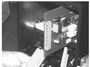
Fig. 55-5 Pull out the plugs of the control boards. Pull out selected control board. Insert new control board
