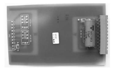
Fig. 19-4c Extinguish capacitor for direct ST supply.
