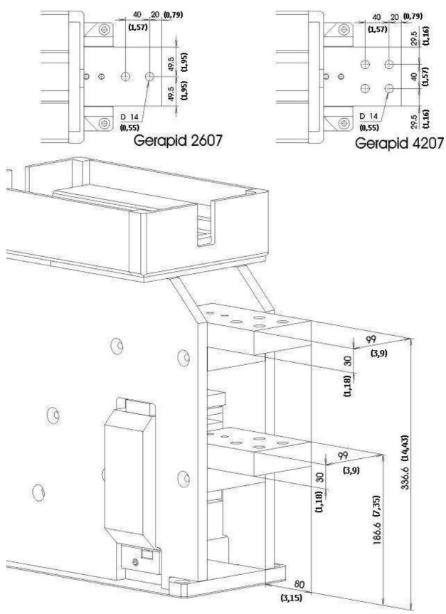
Fig. 36 Gerapid 2607, 4207 with horizontal terminals (dimensions in mm and inches)
