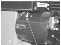
Fig. 2 Contact for grounding wire
