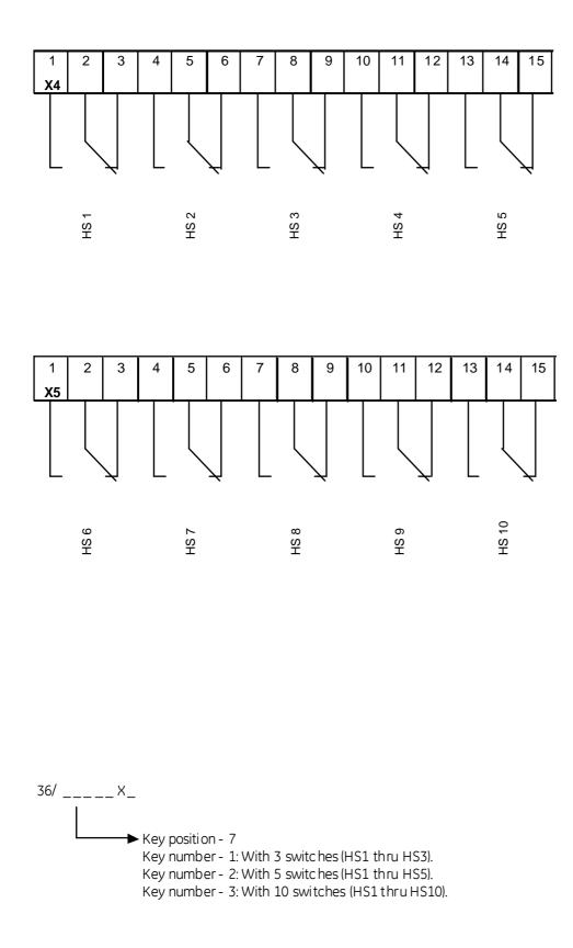
Fig. 30 Auxiliary switch
