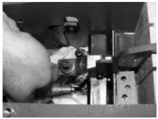
Fig. 52-5 Tighten braid's screws by means of hand
