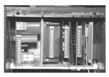
Fig. 54 Control box inside (with SEL unit)
