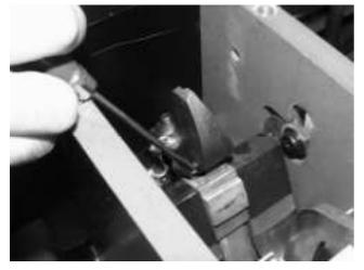
Fig. 52-2 Remove safety ring
