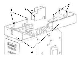
Fig. 43 Adapter and protective walls
