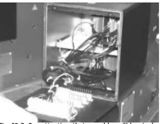
Fig. 55-7 Pay attention, that no cables will be pinched between box and front cover during closing!
