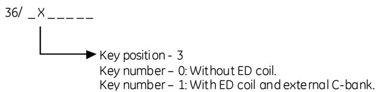
Fig. 24 ED coil with external Capacitor trip device
