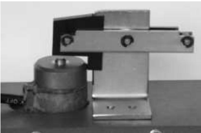
Fig. 8 ED impulse coil with seesaw interface
