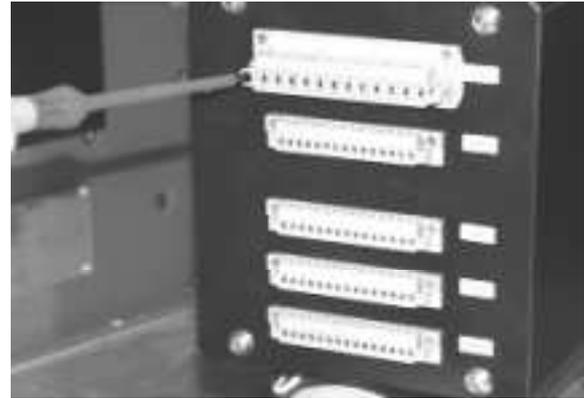
Fig. 55-1 Unscrew and remove all the external plugs
