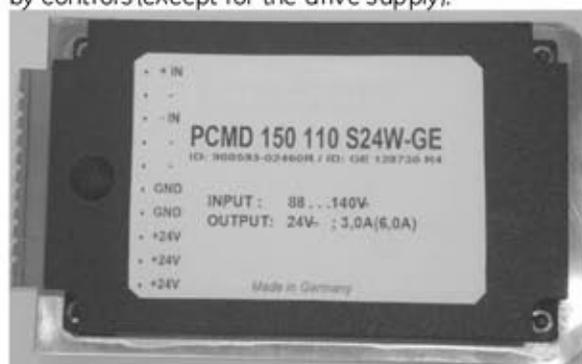
Fig. 19-2 Voltage inverter 110 V/24 V DC.
