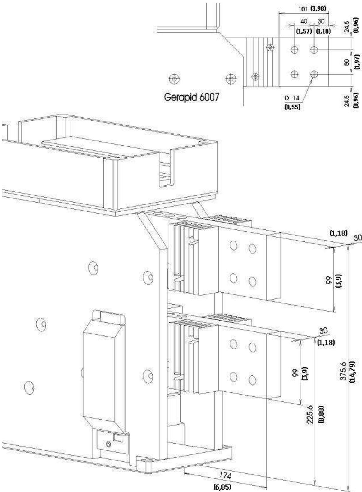
Fig. 38 Gerapid 6007 with vertical terminals (dimensions in mm)
