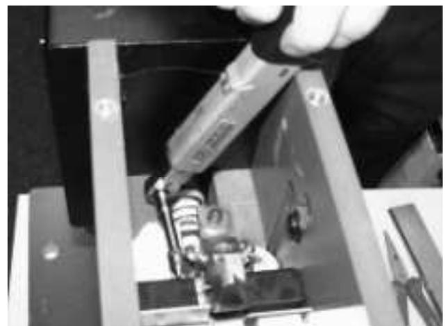
Fig. 52-6 Tighten braid's screw with torque of 10Nm
