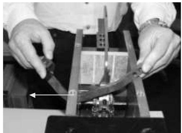
Fig. 51 Taking out the front arc runner of old design
