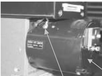
Fig. 2 Contact for grounding wire
