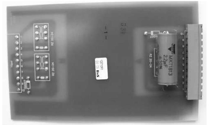
Fig. 19-4c Extinguish capacitor for direct ST supply.
