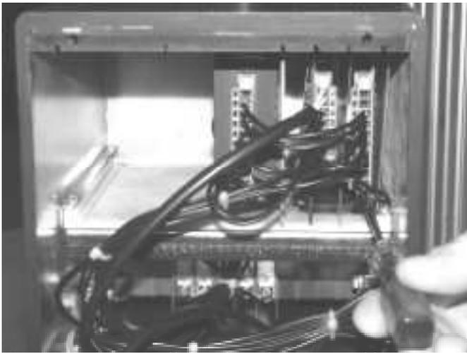
Fig. 55-4 Unscrew all the plugs from control boards
