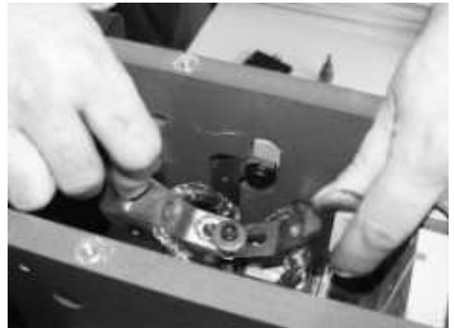
Fig. 52-4 Replace arcing contact
