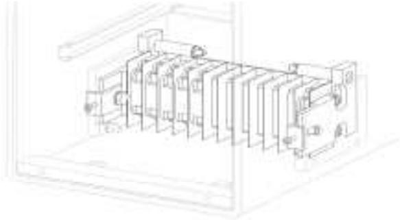
Fig. 12 Auxiliary contacts layout in control box
