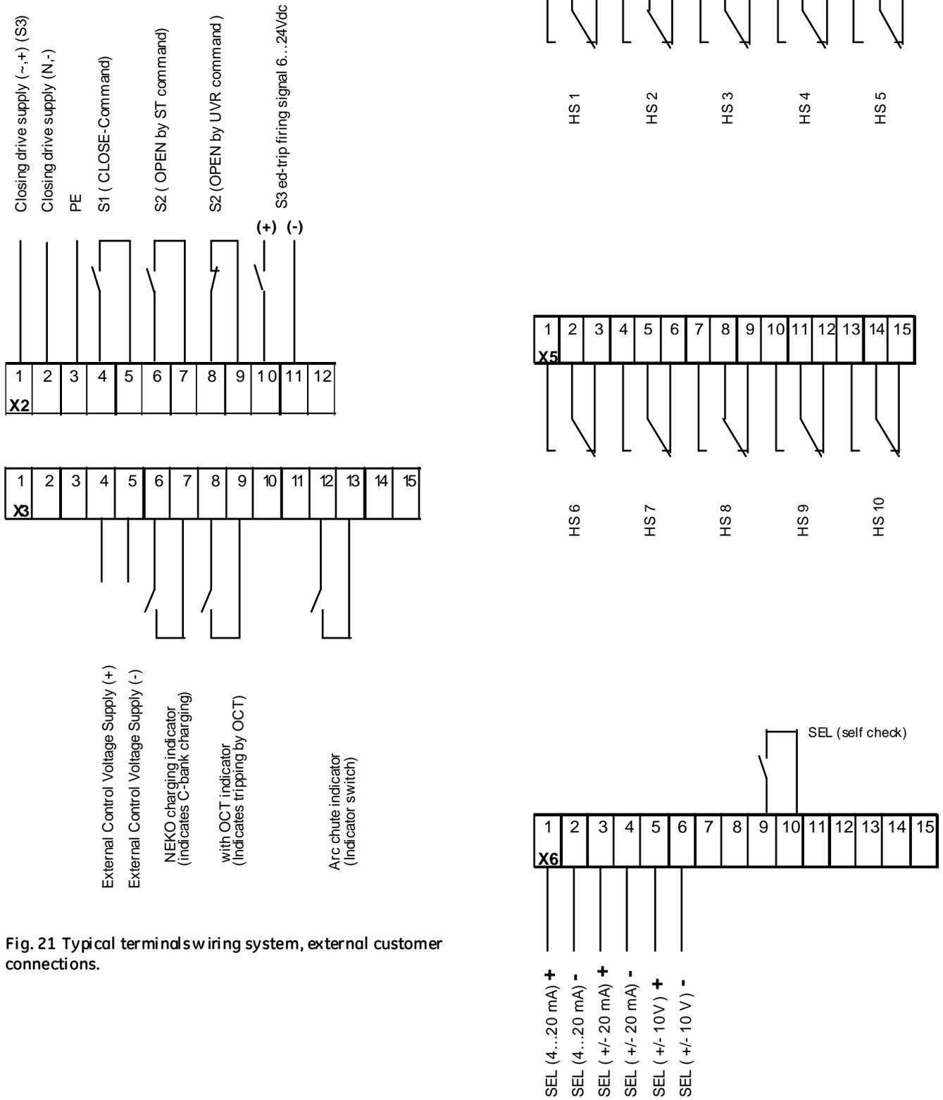
Fig. 21 Typical terminal wiring system, external customer connections.
