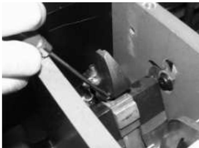
Fig. 52-2 Remove safety ring
