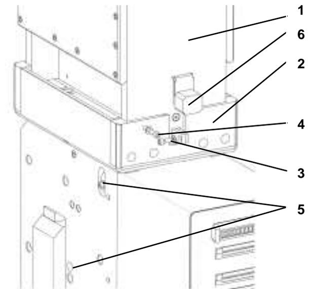
Fig. 41 Arc chute and arc runners fixing
