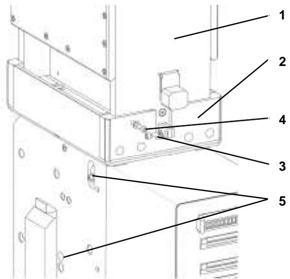
Fig. 49 Arc chute and arc runners fixing
