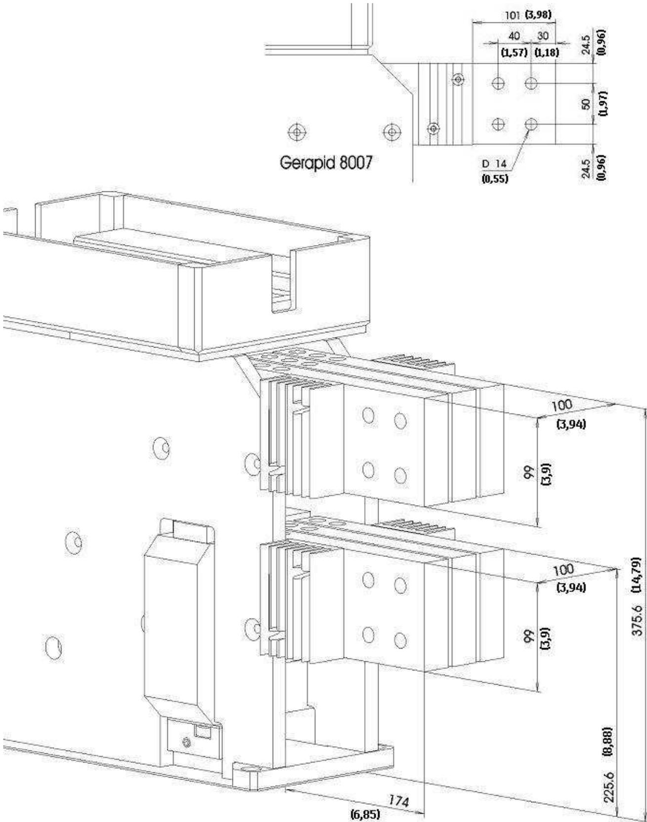
Fig. 39 Gerapid 8007 with vertical terminals (dimensions in mm and inches)
