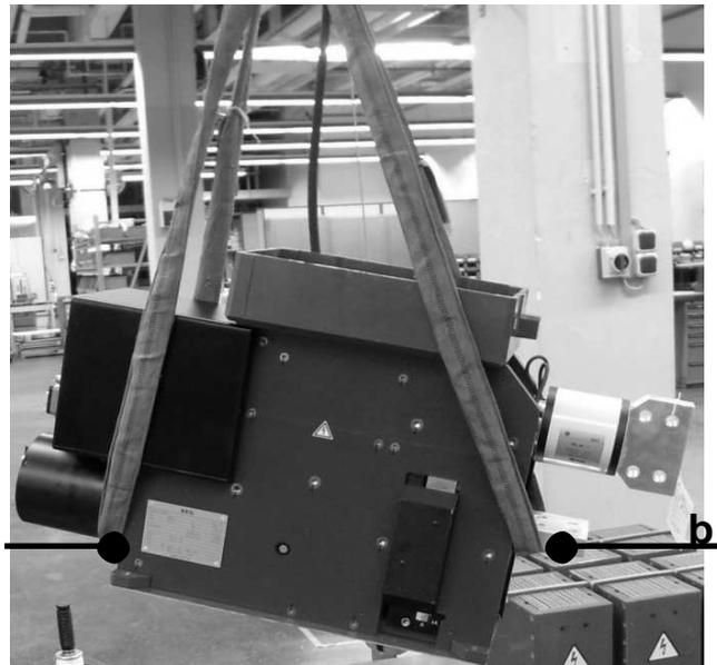
Fig. 1 Handling the breaker
