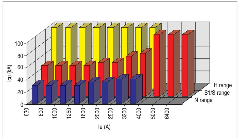
Three ranges of circuit breakers Series ME for time delayed selectivity with different breaking capacities in each frame size offer a compact and economic solution for all installations.
