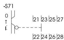
Charged signal for motor-type stored energy
