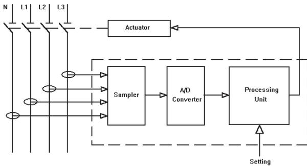
The sampler receives the output signal from the current transformer and transfers the information to the Analog - Digital - Converter. The processing unit analyses the signal and compares the results with the parameter settings. In case of a fault condition, e.g. overload, the activator will be energised to trip the circuit breaker.
