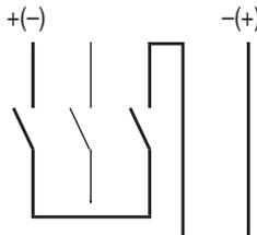
The three pole breaker must be connected in the DC network as shown in the diagram.
