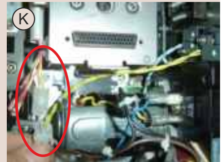
Plug connection CCC-EC switch Steckerverbindung CCC-EC-Schalter Connessione spinotto CCC-contatto CE
