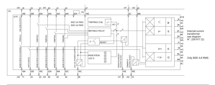
Key position 4 Electronic trip unit type bse 3-7 rms / bse 4-7 rms
