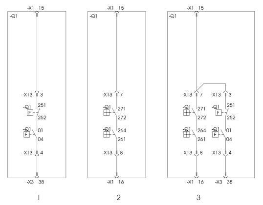
Key positions 11 and 12 Position indication switch at plug-in unit carrier (for further key numbers refer to handling instruction 'withdrawable technique')
