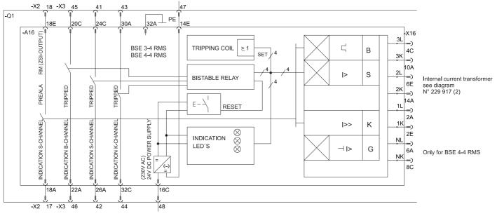
Key position 4 Electronic trip unit type bse 3-5 rms / bse 4-5 rms
