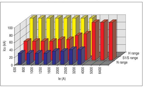
Three ranges of circuit breakers Series ME for time delayed selectivity with different breaking capacities in each frame size offer a compact and economic solution for all installations.
