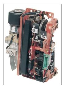
The drive mechanism with an energy storage facility is equipped with integral service facilities for immediate actuation without any additional coupling parts, e.g. through a door cut-out. Opening and closing action of the circuit breaker is made by pushbuttons. A positive operated indicator of the switch position and spring charge condition is provided along with a wide field of visibility to the trip unit.
